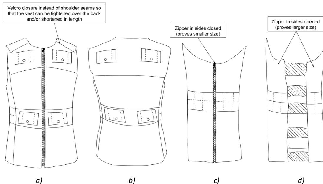
Figure 4. Sketches of prototype vest with sizing solutions, a) front piece with zipper closure, b) back piece c) side piece with closet zipper d) side seam with opened zipper
