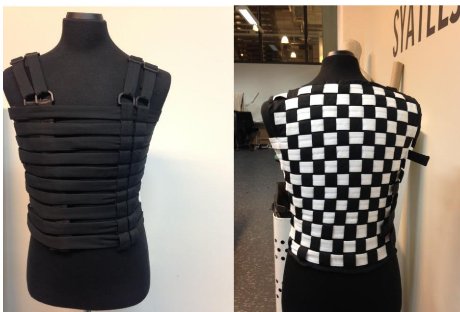
Figure 1. Chessboard vest, D5.7. a) front of vest with straps that can be individually fitted on the person wearing the garment b) back of vest with multiple placement possibilities, actuators are placed on the inside of the vest towards the person wearing it.
