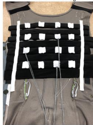
Adjustable velcro (loop) straps with vibration motors attached on velcro (hook) so the placement of the vibration motors can be adjusted in closeness in both horizontal and vertical direction.
