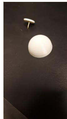
Figure 2. a) The markers placement; b) Markers used are highly reflective semi-spheres.
