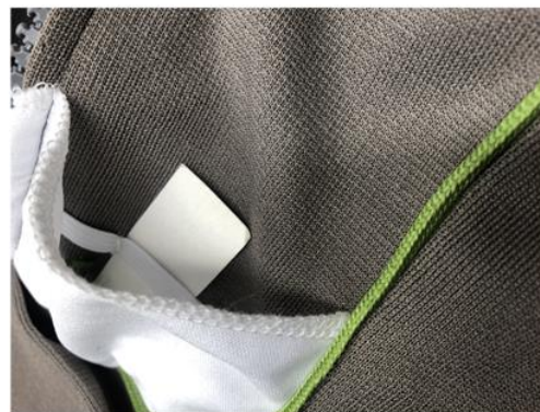
DETAIL - vibration motor placement in pocket
