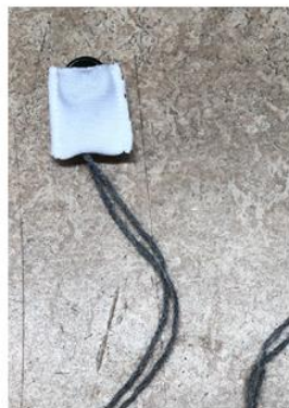
Vibration motor placed inside pocket
