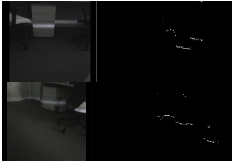
Figure 27: Example of point cloud returned by planar laser scanner.
