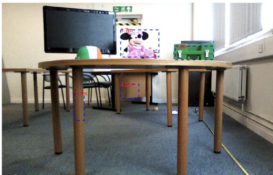
Figure 8: an example of target object distance measurement: once a bounding box for a recognised has been established in the RGB image, it can be projected to the depth image to estimate the distance.
