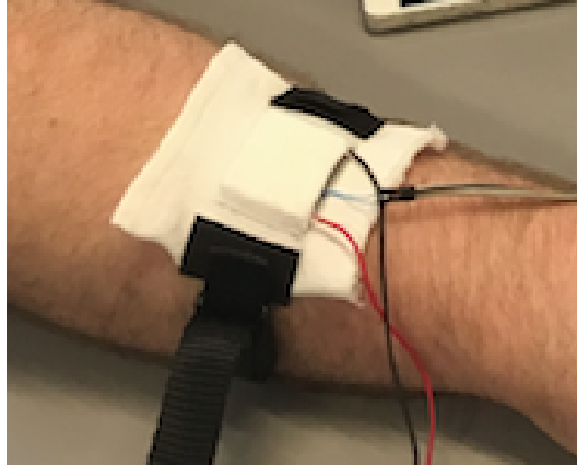
Figure 1: Peltier element in knitted pocket strapped to the skin of the forearm. The Peltier element is concealed by the fabric but is contacted by a red and a black wire. A thermistor (green-blue) is placed below the Peltier element in the pocket.
