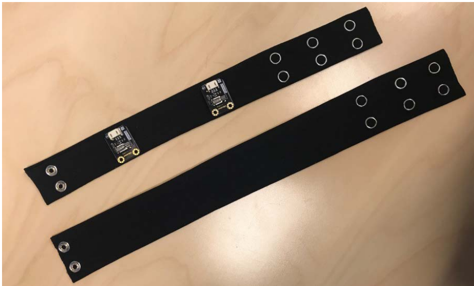
Figure 1: Textile band in female size with VBMs and textile band in male size.
