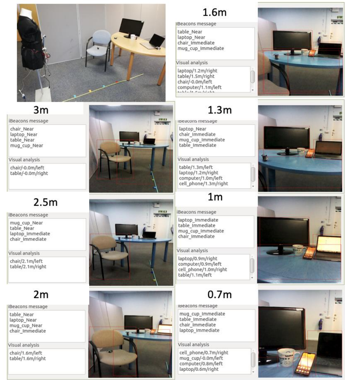
Fig 8: Results of static object detection. Images were captured in the local computer in Leeds, the image color changed due to image display format
